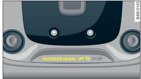
Fig. 64 Headliner: indicator light to display the status of the front passenger's airbag
