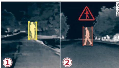
Fig. 97 Instrument cluster: pedestrian marking and warning
