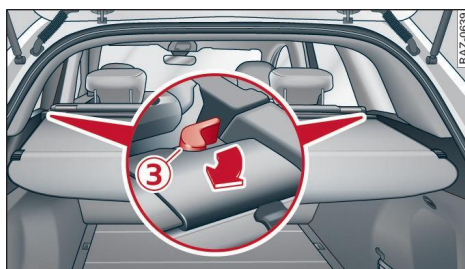
Fig. 72 Luggage compartment: removing the luggage compartment cover
