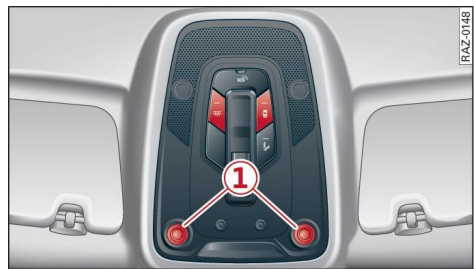
Fig. 38 Headliner: interior lighting
