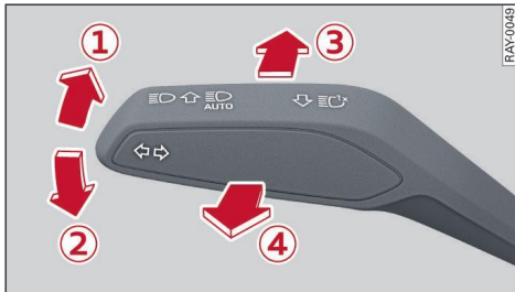
Fig. 36 Operating lever: switching the light functions on and off
