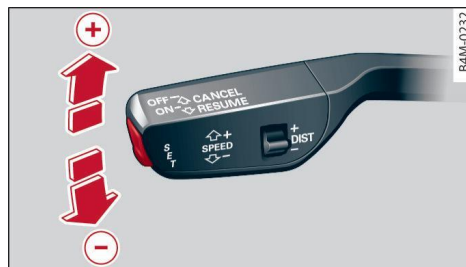
Fig. 103 Operating lever: changing the speed
