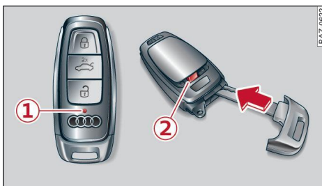
Fig. 26 Vehicle key: removing the battery holder
