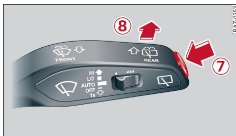
Fig. 44 Lever: rear window wiper
