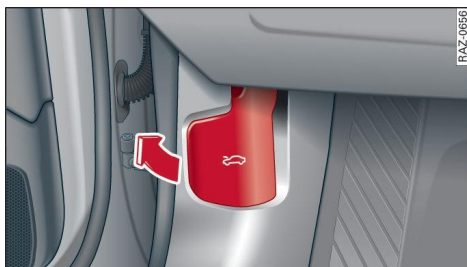
Fig. 156 Footwell: release lever
