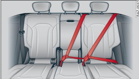
Fig. 68 Rear bench seat: securing unused safety belts
