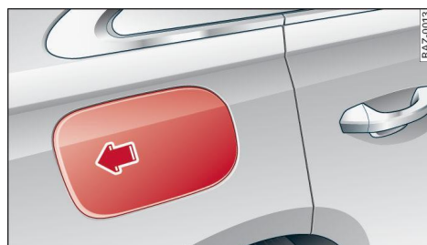
Fig. 154 Right rear side of the vehicle: opening the fuel filler door
