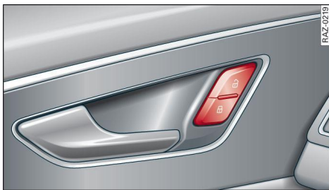
Fig. 21 Driver's door: central locking switch
