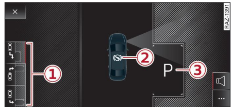
Fig. 130 Upper display: activated parking space search
