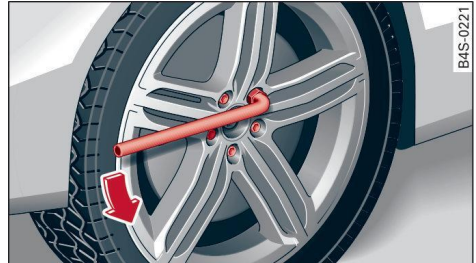
Fig. 175 Wheel: loosening the wheel bolts
