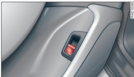
Fig. 28 Driver's door: opening the luggage compartment lid
