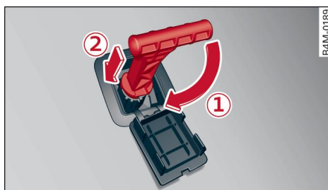
Fig. 87 Footwell: releasing the parking lock using the emergency release
