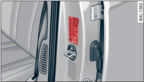
Fig. 167 Driver's side B-pillar: tire pressure label
