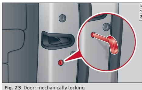
Fig. 23 Door: mechanically locking
