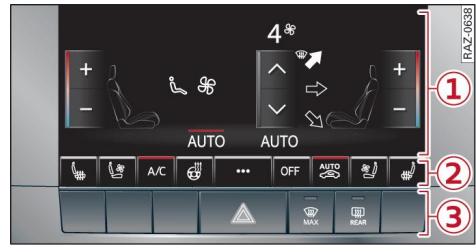
Fig. 81 Center console: lower display and switch panel
