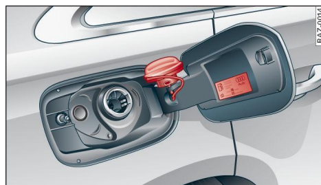
Fig. 155 Fuel filler door with attached fuel cap
