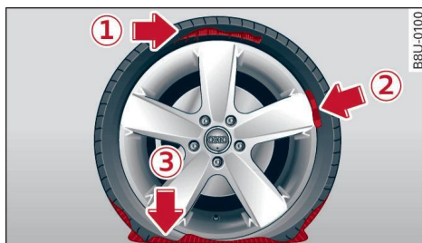
Fig. 170 Tire: tire damage that cannot be repaired
