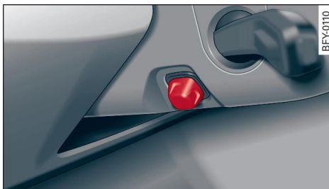
Fig. 54 Steering column: switch for adjusting the steering wheel position
