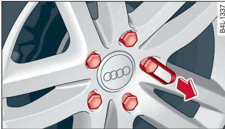
Fig. 173 Wheel: wheel bolts with caps
